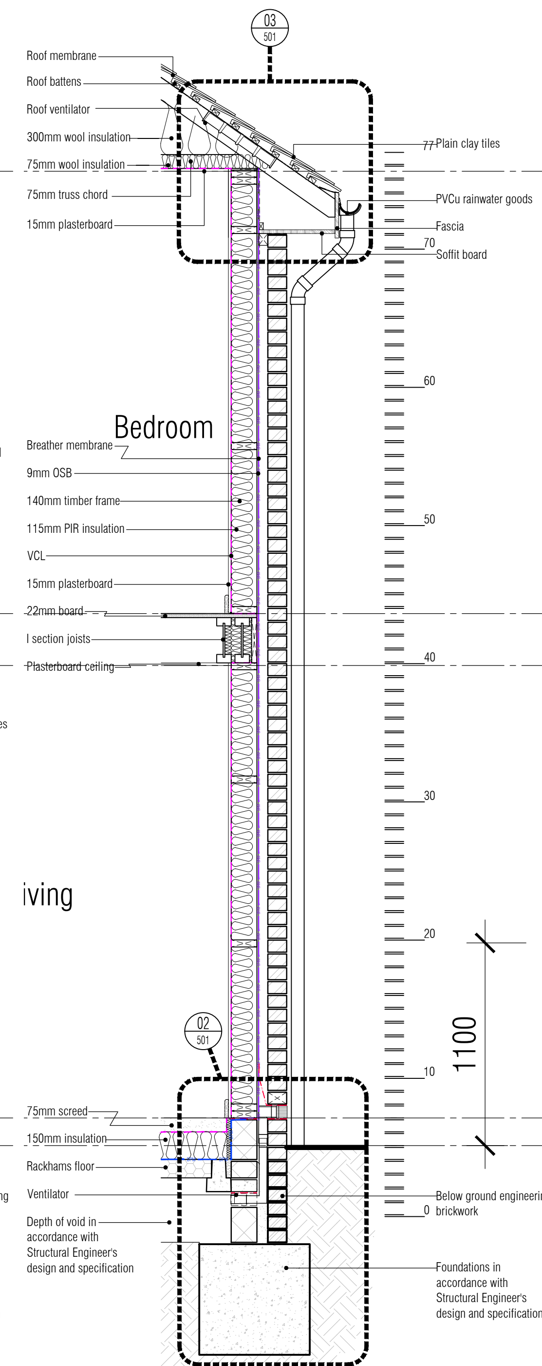
04 Brickwork Strip Section 04 Scale: 1:20
